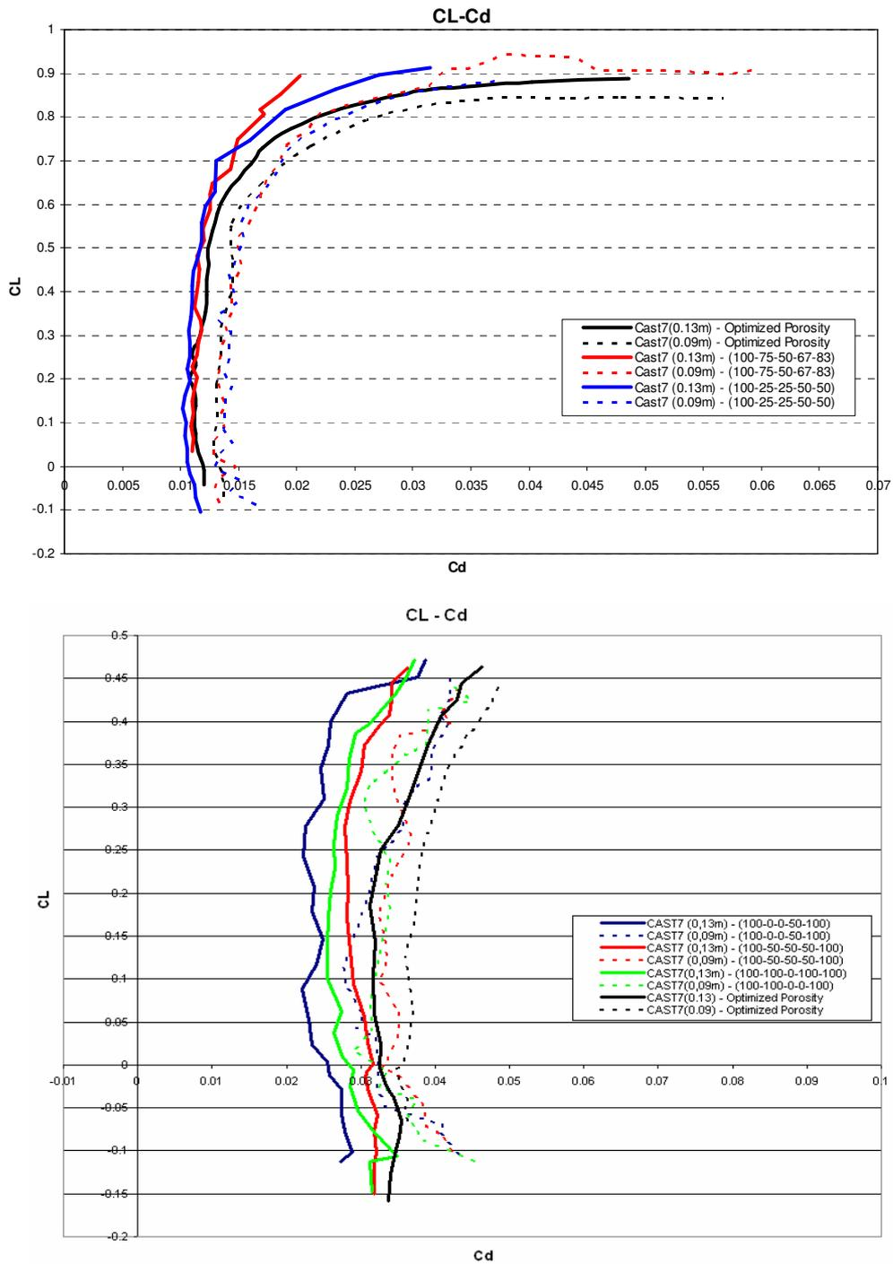
**Figure. 17. Drag curve measured at the optimal porosity distributions on both the small and the large CAST 7 airfoil models at Mach 0.73 and 0.85 compared to a non optimal condition.**
