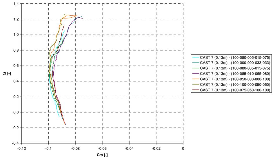
**Figure. 8. Results at M=0.6 on the CAST7: Effects of wall porosity distribution on  $C_d$**
