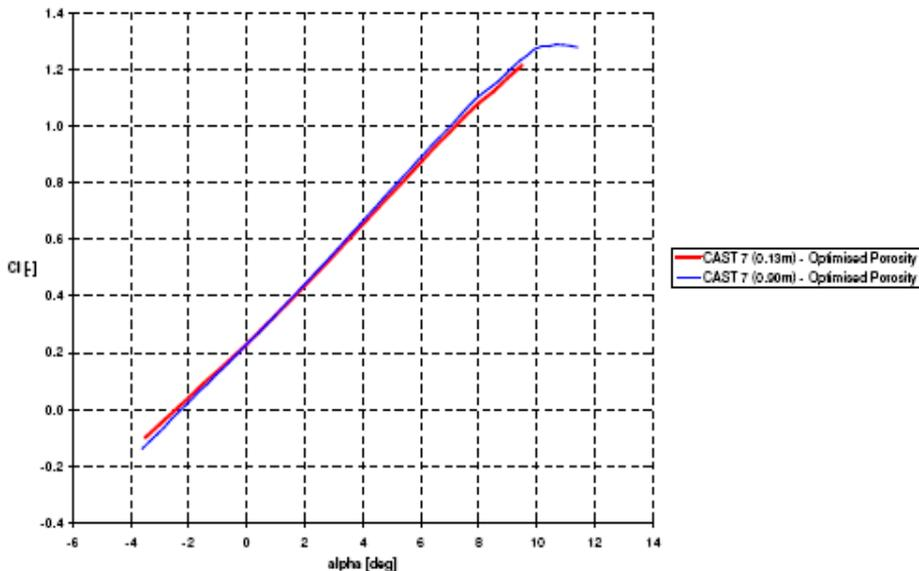
**Figure. 13. Lift curve measured at the optimal porosity distributions on both the small and the large CAST 7 airfoil models at Mach 0.6**
