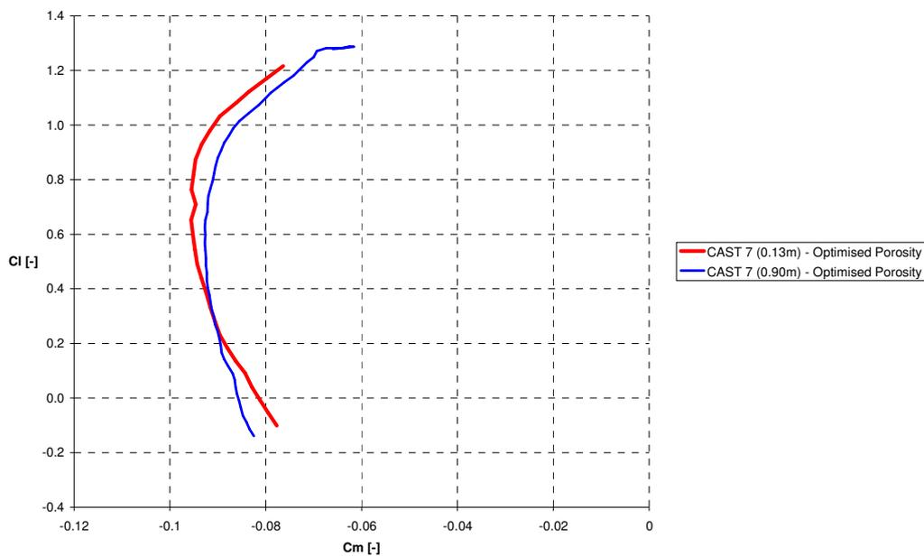
**Figure. 15. Pitching moment curve measured at the optimal porosity distributions on both the small and the large CAST 7 airfoil models at Mach 0.6**
