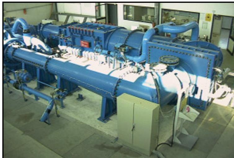
**Figure. 1. CIRA PT-1 Transonic Wind Tunnel**
