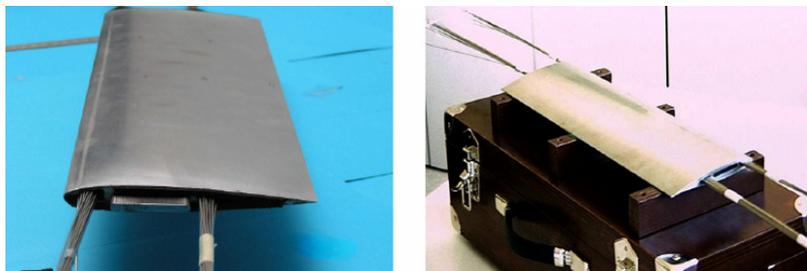
**Figure 3. NACA 0012 airfoil and CAST7 supercritical airfoil**
