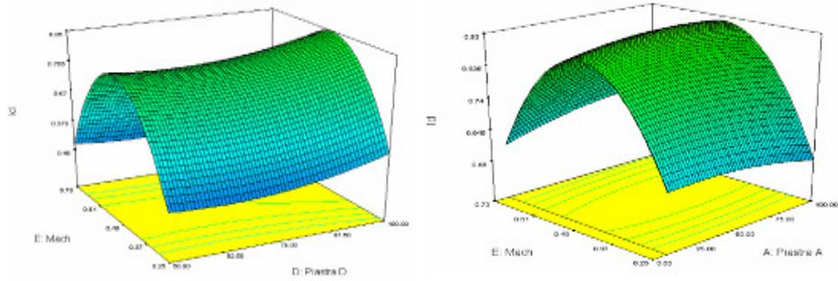
**Figure. 9: Response surface: interference parameter measured on the lift curve as function of the Mach number and the position of first and fourth plates (factors A and D)**
