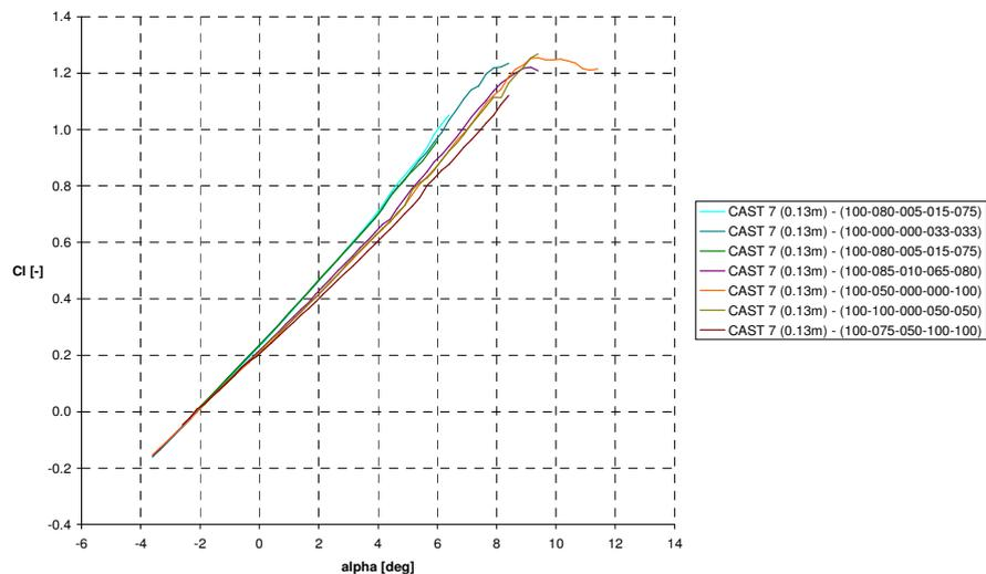
**Figure. 6. Results at M=0.6 on the CAST7: Effects of wall porosity distribution on  $C_l$**
