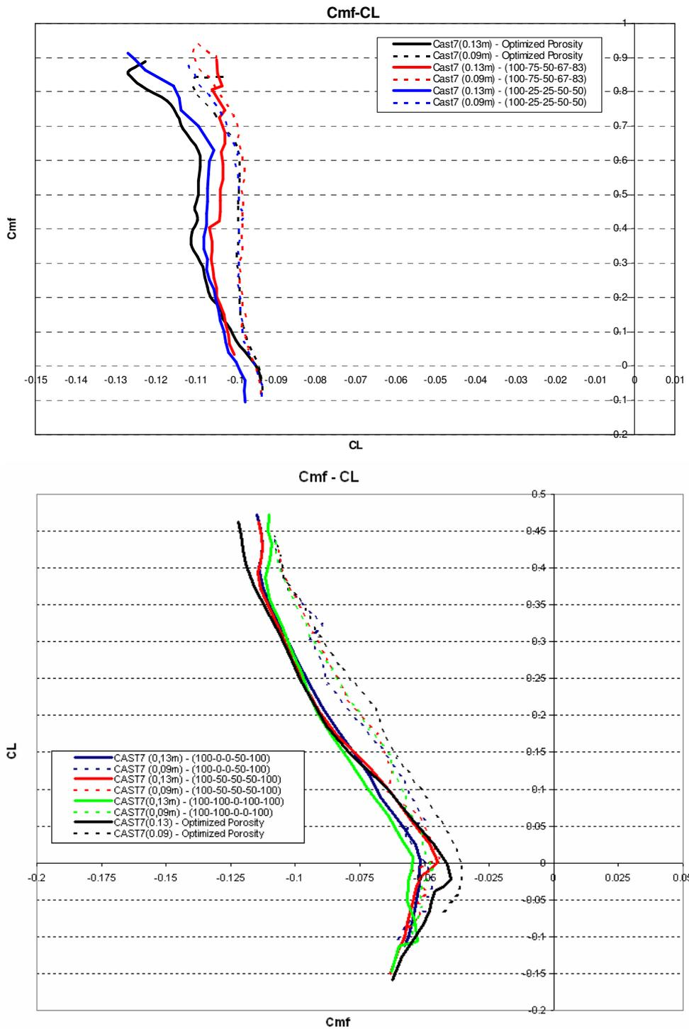
**Figure. 18. Pitching moment curve measured at the optimal porosity distributions on both the small and the large CAST 7 airfoil models at Mach 0.73 and 0.85 compared to a non optimal condition.**
