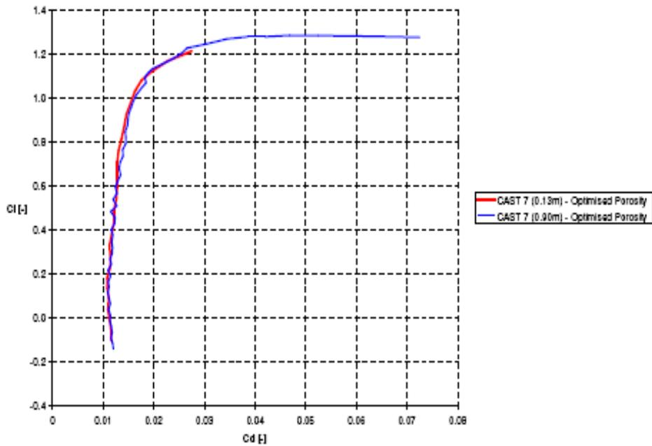
**Figure. 14. Drag curve measured at the optimal porosity distributions on both the small and the large CAST 7 airfoil models at Mach 0.6**
