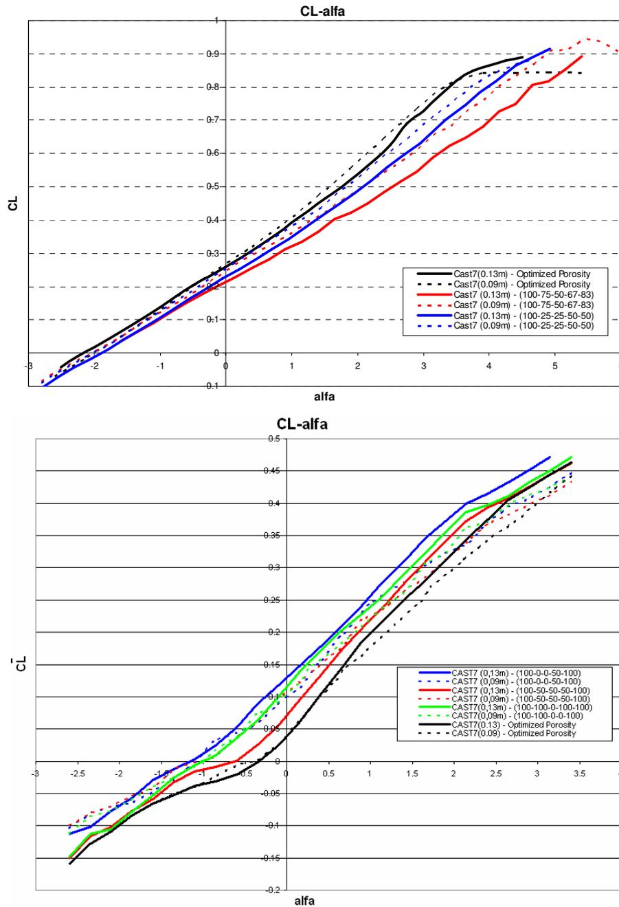
**Figure. 16.** Lift curve measured at the optimal porosity distributions on both the small and the large CAST 7 airfoil models at Mach 0.73 and 0.85 compared to a non optimal condition.
